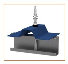
Step 2: Screwing- in hanger bolt on the roof to roof beam.
